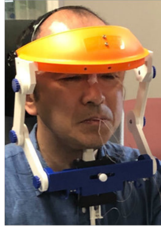
Figure 1: (left) Isometric drawing of the proposed headset. (right) Photo of the proposed probe headset prototype in place. The probe is fixed to the probe clamp with a damper and moves upward and downward following the mandible movements.
